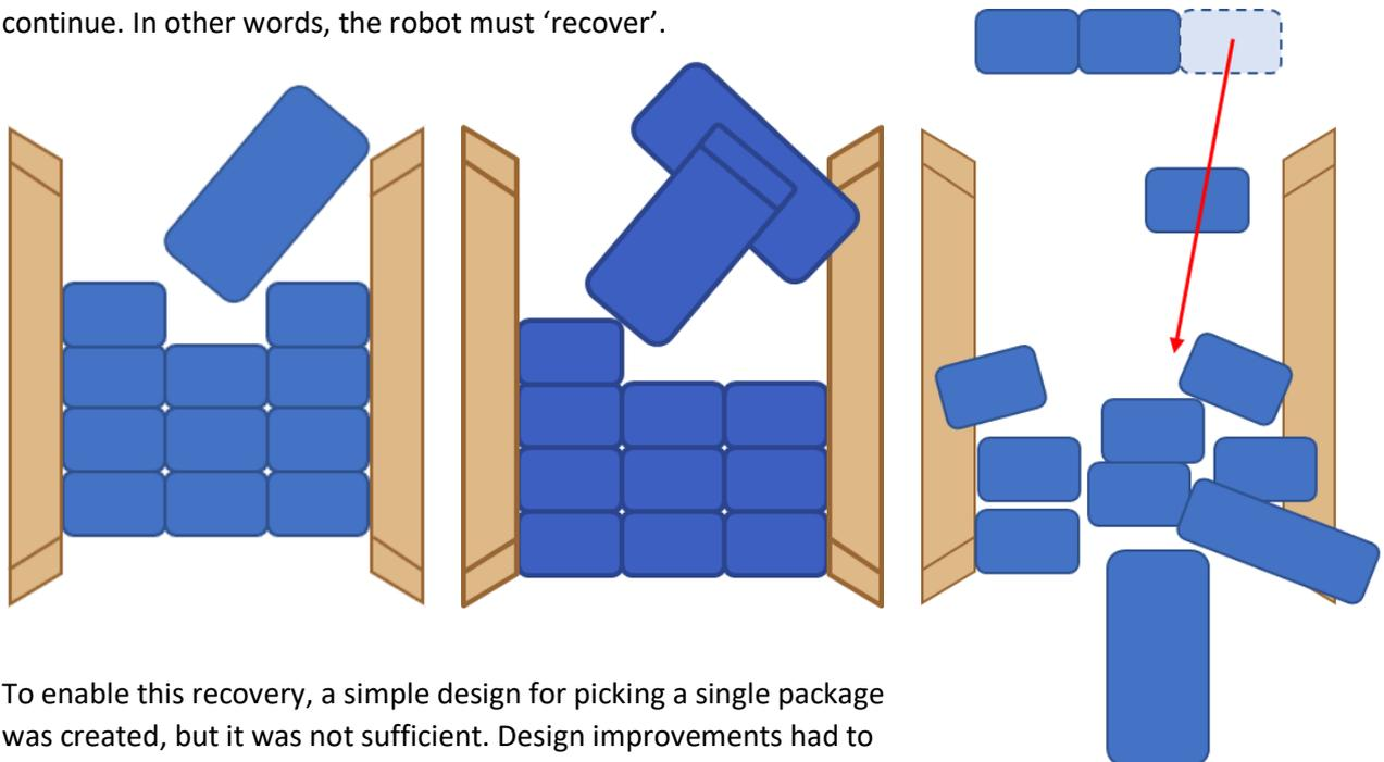
To enable this recovery, a simple design for picking a single package was created, but it was not sufficient. Design improvements had to be made; a longer trunk, a more conformable suction cup and a spring-loaded trunk to not crush packages. Air connections were simplified and hoses designed away, and a hanging mechanism was added to the attachment so that it would not fall of the gripper head if vacuum was not running.
