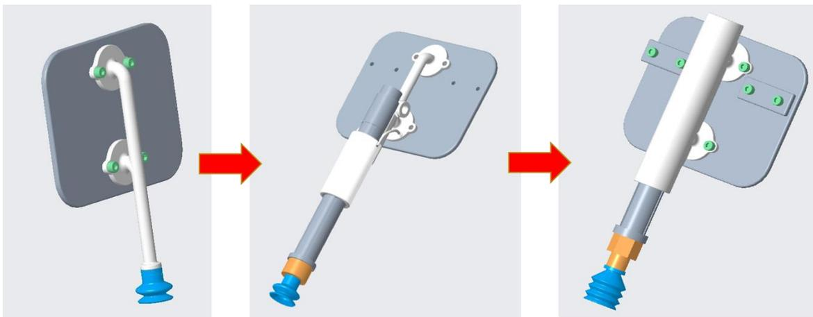
The final picking attachment can be seen in the figure to the right. The design was tested for speed and robustness and showed good results in both aspects. Picking angles of up to 55 degrees were tested and the attachment showed no difficulties in handling these. Picking speeds of down to 1 second per package was measured, but was highly dependent of the package orientation and the travel distance of the package from the pick-up point to the drop point.
